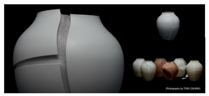
When touched, the Shape Memory Sheet softens at normal temperature and gradually returning to its original shape.
