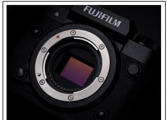
New back-illuminated 40.2MP X-Trans™ CMOS 5 HR sensor
