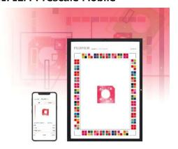
An app designed for use with the pressuremeasuring film "Prescale." The app allows users to easily quantify pressure by capturing a color-developed "Prescale" with a mobile device, and enables further data use by connecting the app with a dedicated cloud system.
